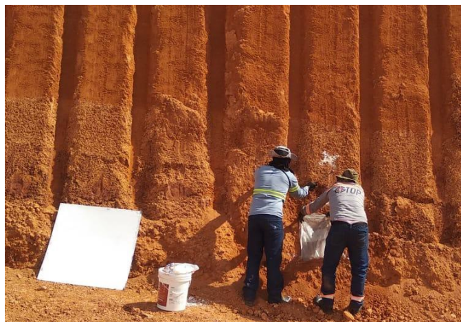
Figure 5. Sampling at pre-defined points for laboratory analysis.
