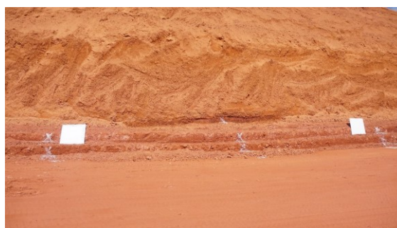
Figure 4. Imaged slope showing standard barium sulfate plates and locations (X markings) from where samples were taken for laboratory analysis of mineral content.
